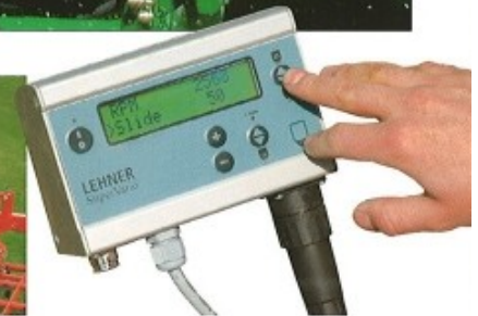
Digital in-cab control with easy set-up and operation for easily adjustable spread width and application.
