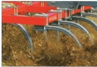
Heavy duty double leaf 'C' tines with heavy duty forged reversible points provide optimum operating angle and efficient penetration.
