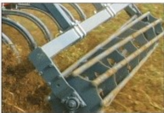
The cultivating depth of the tines is controlled by an adjustable 400mm diameter rear mounted crumbler roller. This levels and consolidates the surface and crushes clods.
