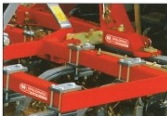
The cultivator's main frame is manufactured from 100mm square profile steel for strength and durability.
