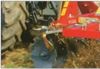
De-mountable multi-disc headstock provides adjustment of disc cultivation depth – independent of the tine depth.
