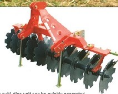
The multi-disc unit can be quickly separated from the cultivator and used – via a three point linkage – in conjunction with any cultivator or be mounted on a tractor front linkage.
